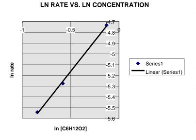
If we plot the natural log of the concentration vs. the natural log of the rate we get a slope = 1.14, and therefore the order of the reaction is 1.14 as well.
